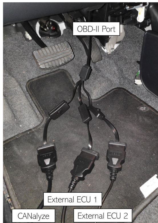
Figure 6.2: Using an OBD-II port splitter in the ATLASCAR2 to connect all the devices to the vehicle's network.
