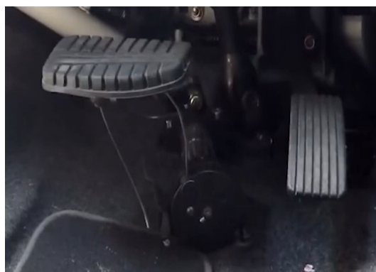
Figure 2.3: Remote control solution for the braking system in the AUTO C-ITS project in Madrid.
