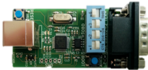
Figure 3.1: CANalyze - open source hardware to receive and transmit CAN messages [23].
