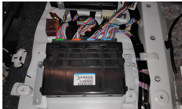
Figure 3.3: Control unit responsible for the propulsion operation in the ATLASCAR2.
