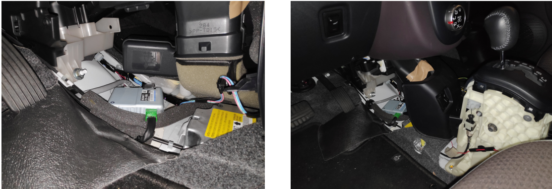
Figure 3.2: Control unit responsible for the steering operation in the ATLASCAR2.
